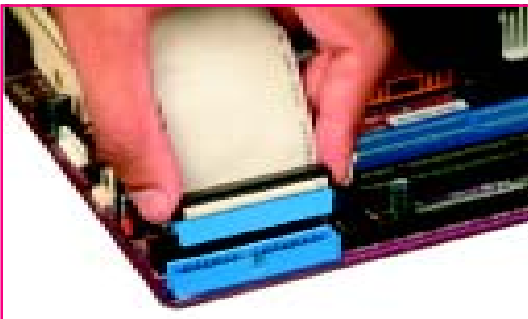
Figure 10-11 Connecting IDE cable to IDE port
